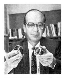
COUNTER AND TIMER using magnetically set wires to perform switching function are displayed by inventor Gordon Bachand (7261). He plans application of the device to magneto-optic memories.
